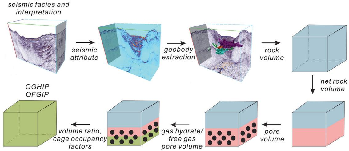
**Fig. 4. Schematic diagrams of in-place gas resource assessment. Three-dimensional reservoir extent is calculated based on geobody volume extraction. OGHIP: original gas hydrates in-place; OFGIP: original free gas in-place.**
