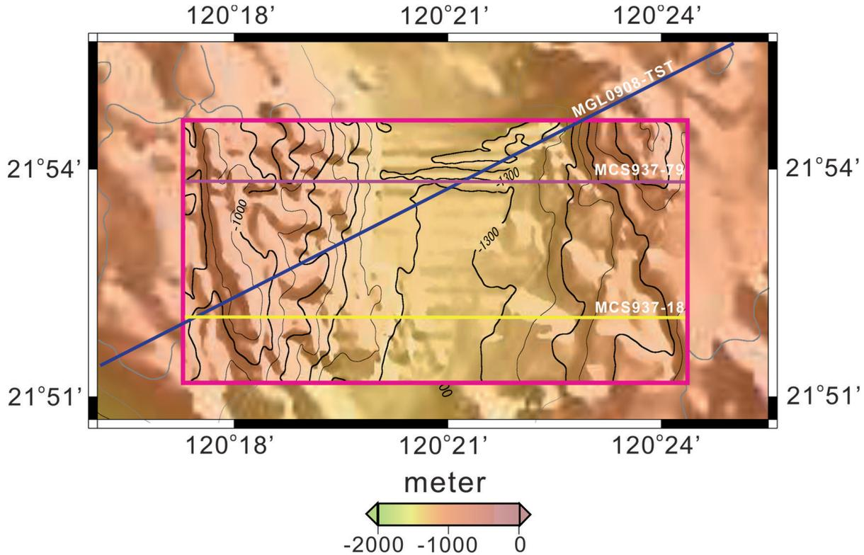
**Fig. 5.** High resolution seafloor image from the MCS937 3D seismic volume (pink square) superimposed on bathymetry data. Profiles of the three interpreted seismic lines, MGL0908-TST, MCS937-79 and MCS937-18 are shown by the dark blue, purple and yellow-coloured lines, respectively; the interpreted profiles are presented in Figs 7, 8 and 9.
