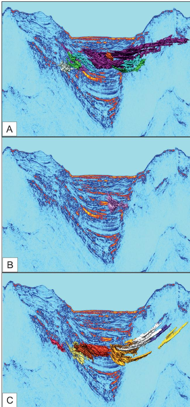
**Fig. 12. Geobody extraction based on amplitude-driven attributes for (A) gas-hydrate compartments above BSRs, (B) free gas compartments above BSRs and (C) free gas compartments below BSRs. The geobody colours represent different voxel volumes generated from amplitude opacity.**
