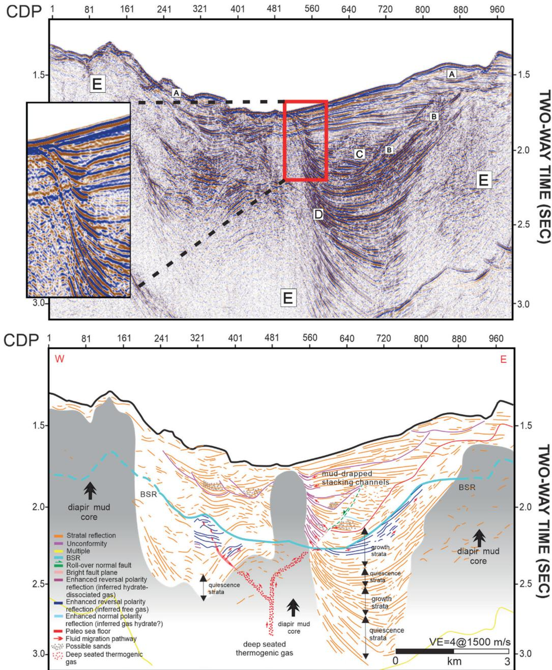
**Fig. 9. Uninterpreted (above) and interpreted (below) reflection seismic profile from the MCS937-18 2D line. The inset, uninterpreted figure is an enlargement profile (red square), showing dragged reflections on the diapiric flank with reversal polarity. Similar reflection characteristics are seen below the BSRs. Abbreviations: CDP, common depth points; VE, vertical exaggeration. Letters in the uninterpreted figure indicate facies types (see Table 1).**
