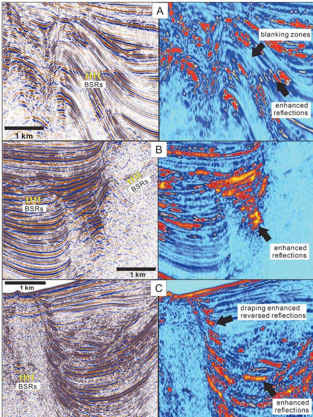
**Fig. 11.** Comparison of conventional seismic and envelope attribute profiles for (A) MGL0908-TST, (B) MCS937-18, and (C) MCS937-79. Together with phase information, the attribute was used to delineate free gas and gas-hydrate bodies. Blanking zones are present above the BSRs and also commonly occur below BSRs; enhanced reversed reflections are also visible above BSRs.
