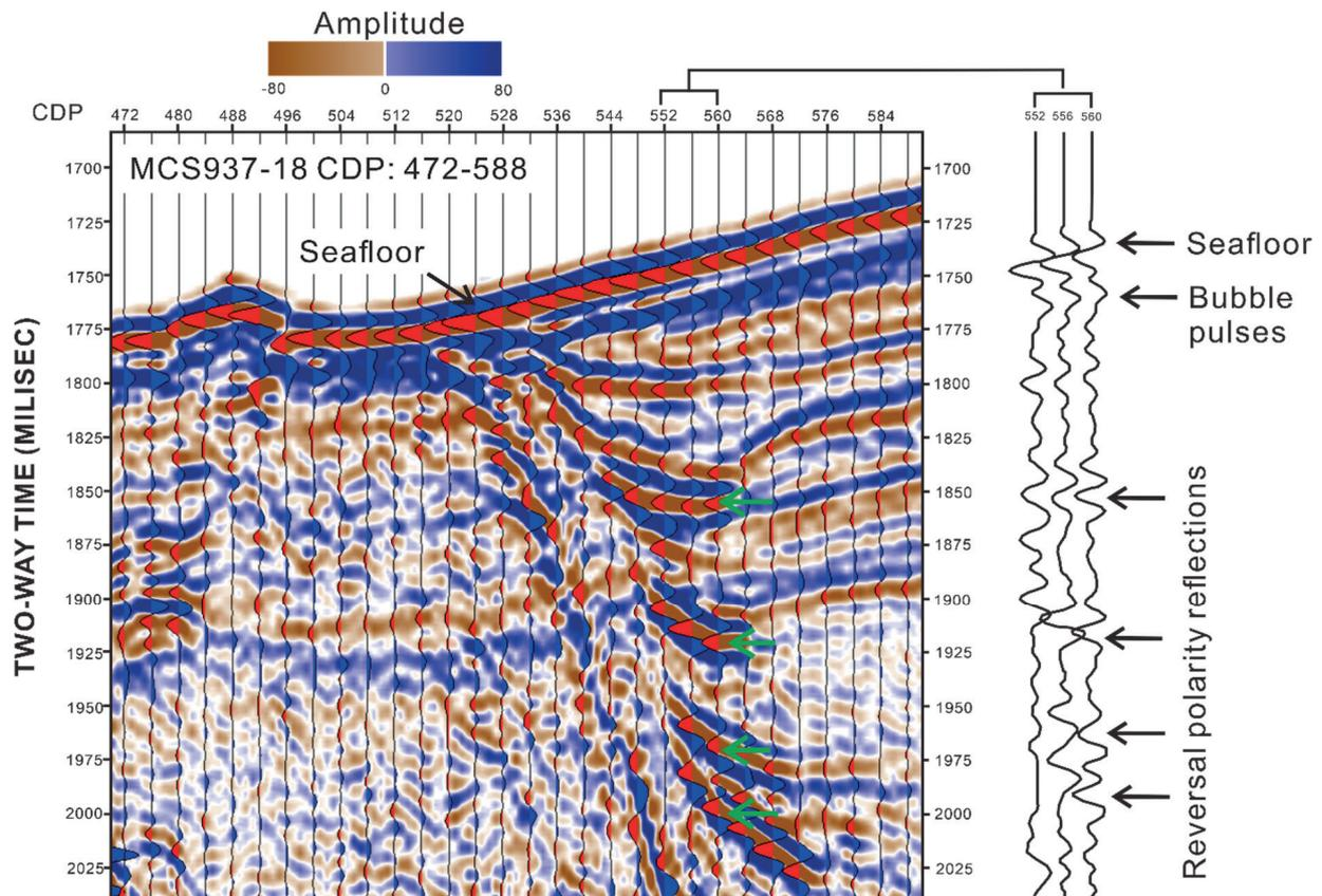
**Fig. 10.** A segment of seismic profile MCS937-18 in the study area, showing enhanced reflections draping on the dome-shaped reflections (green arrows). Amplitudes with blue colour represent positive reflection coefficients, and those with red colour indicate negative reflection coefficients. The extracted wavelets on the right show seismic amplitudes and associated interpretations. Note that the phase of the enhanced reflections is reversed relative to that of the seafloor.
