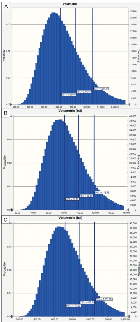
**Fig. 13. Probabilistic distribution of in-place gas volumes for (A) gas-hydrate compartments above BSRs, (B) free gas compartments above BSRs, and (C) free gas compartments below BSRs in the study area.**
