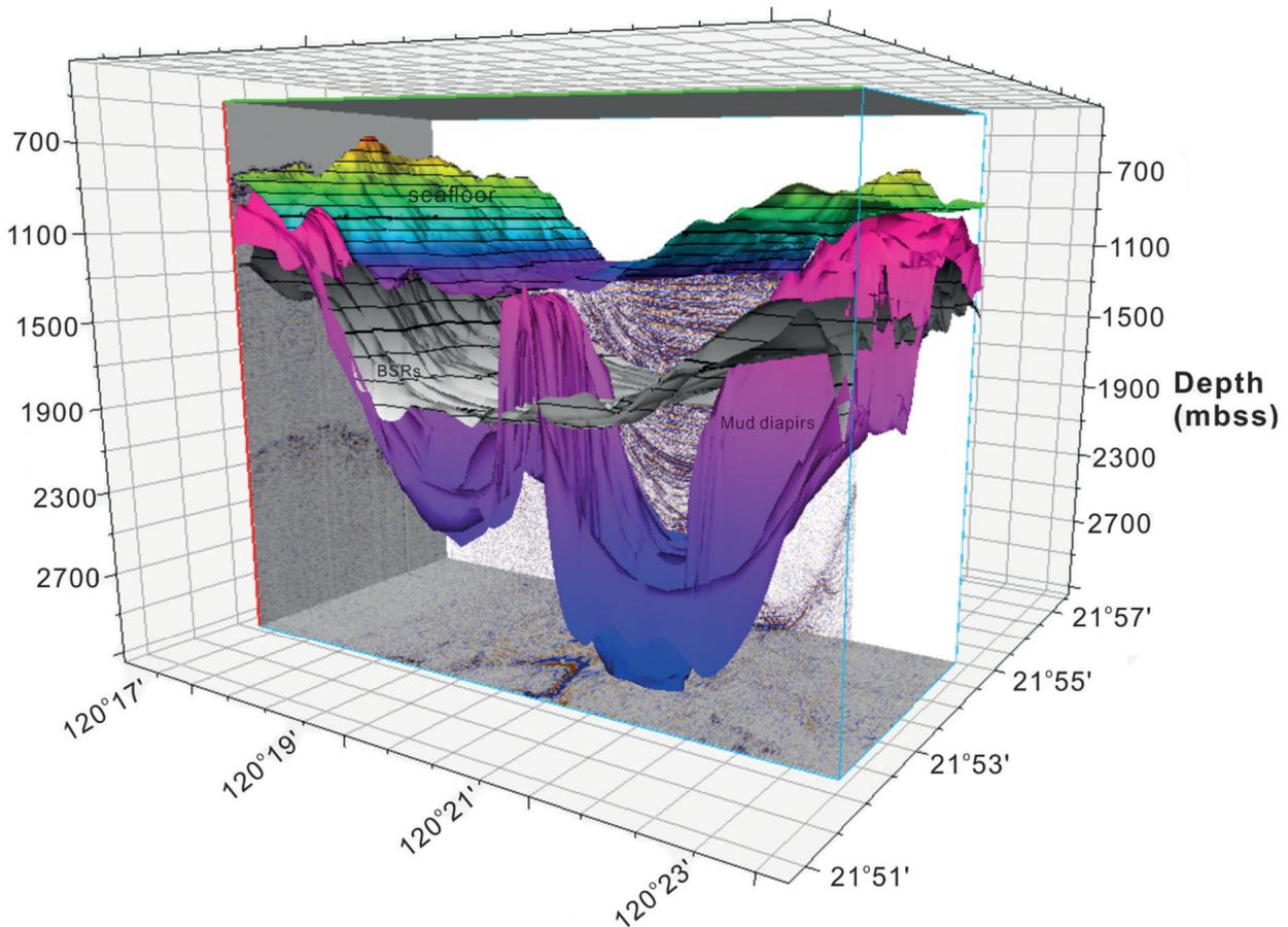
**Fig. 6. 3D block diagram combining three-dimensional seafloor bathymetry, BSRs and mud diapirs. BSRs are clearly imaged across the mud diapirs. Abbreviation: mbss: metres below sea surface.**
